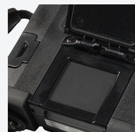
FAP 45 fingerprint sensor
